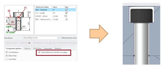
A rule set for chamfer sizes can be defined in EMX options.
