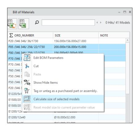
Reset the model size to the current parameter value for selected components from the Right Mouse Menu:
