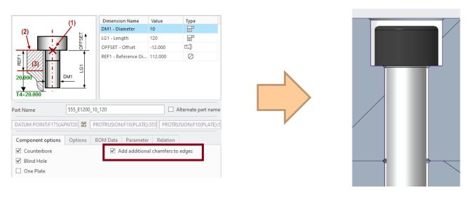
A rule set for chamfer sizes can be defined in EMX options.
