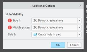
If at least one part is found that must not be changed, the user must enable the creation of the hole in the 'Additional Options' dialog.
